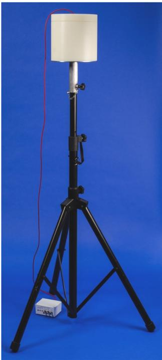
The NNS is the long-awaited, simple solution, for the routine field use of the well-known Bonner Sphere method. At the heart of the NNS are 7 moderating cylindrical shells, placed one inside the other, providing a lighter-weight compact instrument for neutron field characterization.
